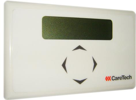
The CareTech dementia monitor can be connected to the Gustav tracking beacon and the patient wears an alarm pendant hidden inside the pendant is an RFID device which will automatically send a location at a preset time.
